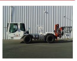
The unit has 500 liters load capacity of AN-FO, with the possibility of incorporating a crane and basket that completes, even more, its usefulness in mining.
