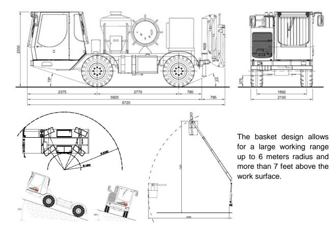
TRANFOX-500 is equipped with all the elements to make easy a hard work: Rotary driving place, ROPS-FOPS cabin, working lights, etc. A full accessibility to high rotation components, make its use and maintenance not a loss of time, but, using it properly, the reason for a long-lasting and reliable unit. The powerful engine allows it to work without loss of power up to 5,000 MASL and to overcome slopes up to 30% full load.
