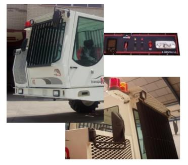
The dumper has a load capacity of 10,000 kg (7 m³). Possibility of incorporating a crane and basket in standard platform that completes, even more, its usefulness in mining.
