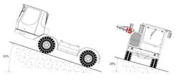
is equipped with all the elements to make easy a hard work: Rotary driving place, ROPS-FOPS cabin, working lights, etc. A full accessibility to high rotation components, make its use and maintenance not a loss of time, but, using it properly, the reason for a long-lasting and reliable unit. The powerful engine allows it to work without loss of power up to 5,000 MASL and to overcome slopes up to 30% full load.
