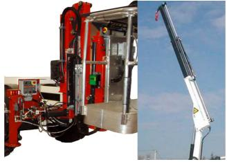
The unit has a load capacity of 10,000 Kg, with the possibility of incorporating a crane and basket that completes, even more, its usefulness in mining.
