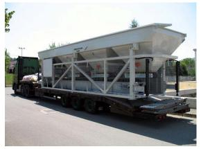
For transport and shipping, the top end of bucket conveyor belt can be swiveled down to the hoppers for reducing the height. Thanks to the four hydraulic stabilizers (optional) can be unloaded from the means of transport and can be installed on the suitable place with no need of a crane.
