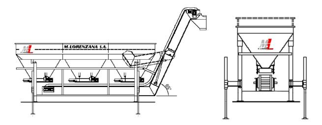
The equipment is provided with an electronic weighing system with digital panel and controlled by automatic programs, which allows us to discharge the pre-selected amount of the different aggregates loaded into each hopper, depending on the type of concrete we want to produce.
