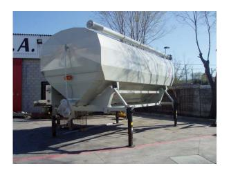
Very Handy and versatile horizontal portable silos for storing and weighing cement which are easily placed on an even surface on the ground, adapting their four telescopic and extendible stabilizers for a perfect leveling, with the aid of concrete or a piece of wood.
