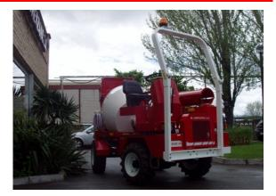
The smallest self-loading mixer in our range of production, *Premier 1A* has an actual output capacity of 1m , accomplishing all safety and robustness of our equipment.
