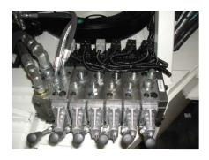
The by arm is operated from hydraulic block and from remote control, equally by radio or cable.
