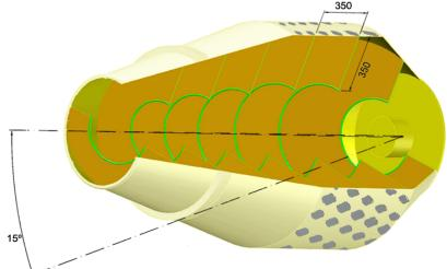
The special internal design of the mixer allows the unit a mixture of dry mass, pouring the water from its own tanks for producing the concrete, or ready wet mix, giving unique smooth finishing features in its sector.
